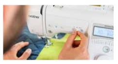
**Speed slide control** The simple slide control adjusts the sewing speed from slow to fast.
